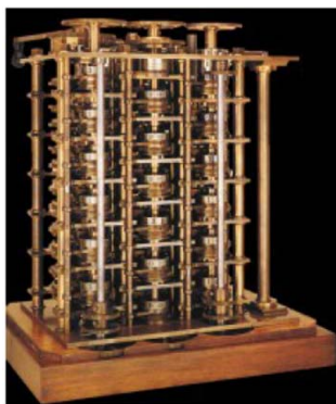
Babbage's Calculating Engine (1833)
