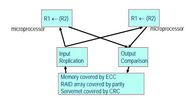
Replicated Microprocessors + Cycle-by-Cycle Lockstepping
